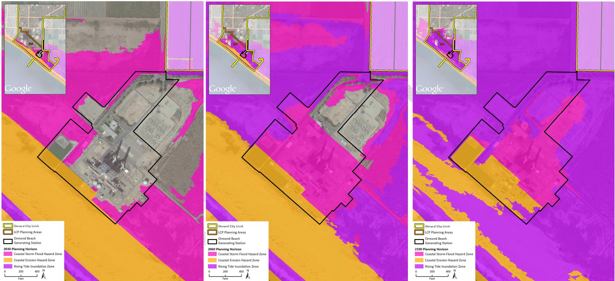
Figure VII-25. Vulnerability of the Ormond Beach Generating Station (OBGS) by Coastal Hazard
