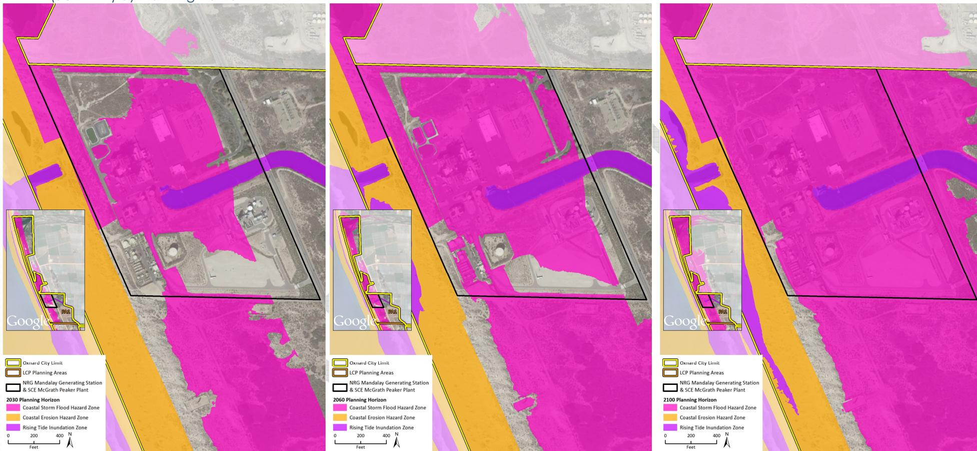
Figure VII-23. Vulnerability of the NRG Mandalay Beach Generating Station (MBGS) and the Southern California Edison McGrath Peaker Plant (SCE MPP) by Coastal Hazard
