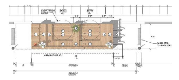
A floor plan showing the existing street, sidewalk, adjacent parking spaces and parklet floor layout and design. Floor plans must be drawn to scale (by hand or computer) and shall contain the following information:
