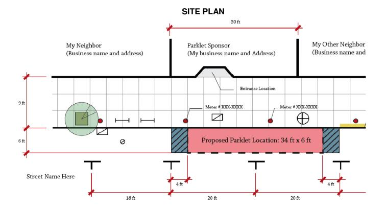
A dimensioned site plan showing the existing street, and sidewalk, and incidental equipment, utilities, etc, is required with all applications. The site plan should show the footprint of the proposed parklet, all street and sidewalk elements at least 20 feet on either side of the proposed parklet location. Site plans must be drawn to scale (by hand or computer), and shall include the following:
