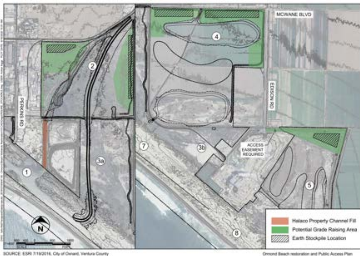
Figure 7-3 Potential Fill and Stockpile Locations
