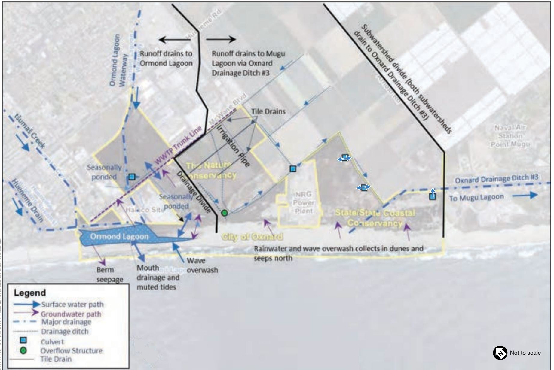
Figure 2-8 Schematic of Surface and Groundwater Flow Paths through the Project Area
