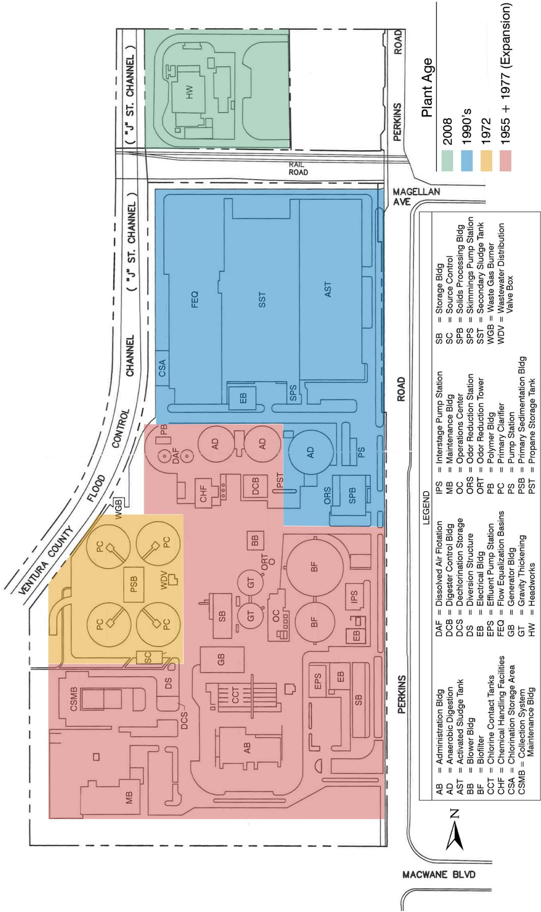
Figure 7. The Oxnard Wastewater Treatment Plant consists of preliminary, primary, and secondary treatment, effluent disinfection and solids handling facilities.
